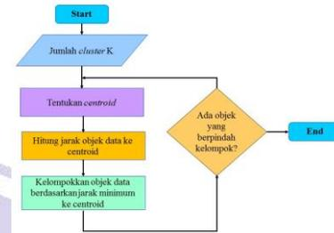
Gambar 2.3 Flowchart Algoritma K-Means Clustering
